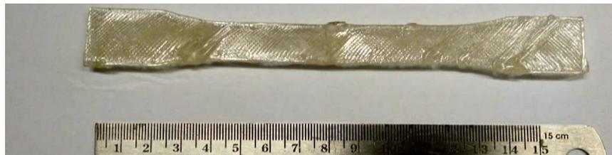
Fig. B: 3D Printed PETG part
