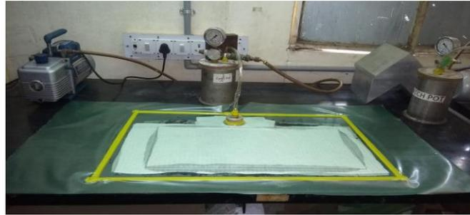
The same process is used for making the composites of carbon prepreg. Here we do not use the resin because the resin is already present in this. For fabrication of thick composite plate, we use debulking process. The debulking process basically, we produced Vacuum in the intermediate step of fabrication. It is used because when we need a thick composite plate then during the process there may be some air left between the layers so to reduce we use this process.
