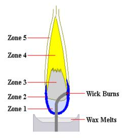
Zone 1 (Non-Luminous Zone) - Fuel on the wick evaporates. There is insufficient oxygen for fuel to burn. Temperature is about 600°C near the wick.
