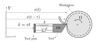
Figure 1: Schematic of single-degree-of-freedom orthogonal turning. The tool post moves with a constant velocity v and its position is represented by  $\tilde{x}$ . The tool tip position at current time is at x(t) and its position before one revolution was at  $x(t\tau)$ .
