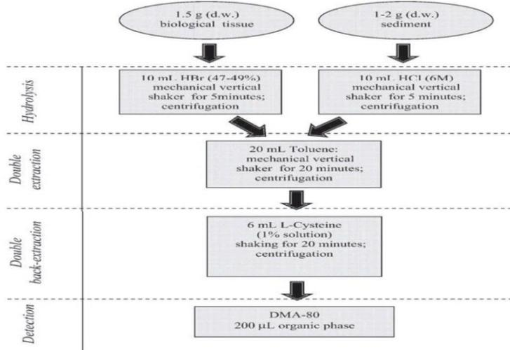
**Fig. 1.** Scheme of the proposed method for MeHg analysis in sediment and biological tissues.
