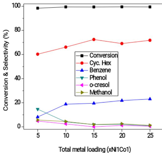
Fig 2. Effect of total metal loading on guaiacol conversion
